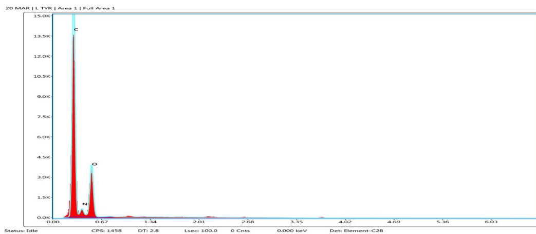
Figure S16: Energy dispersive spectroscopy graph of L-tyrosine
